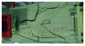
Figure 14 Diagonal cracks in the flange from the experimental program – top view
